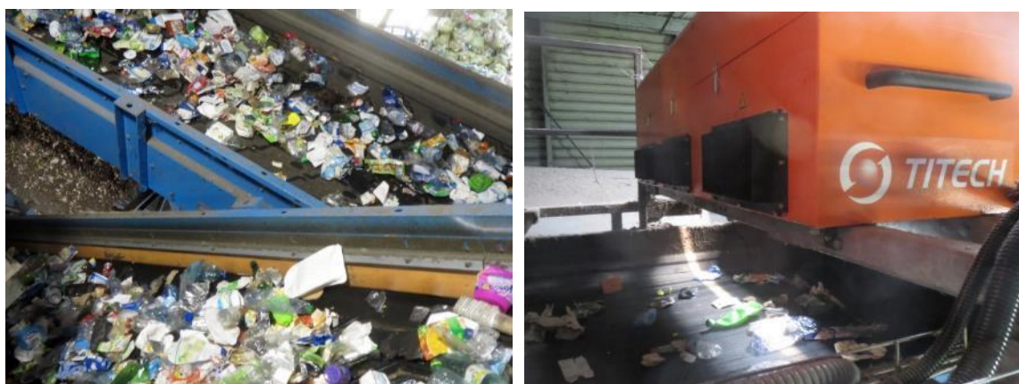
Figure 77: Mouzeuil-Saint-Martin sorting plant – NIR sorting of middle-size fraction
