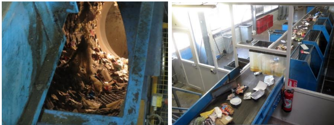
Figure 76: Mouzeuil-Saint-Martin sorting plant – drum sieve generates three different size fractions; large-size fraction sorting is manually
