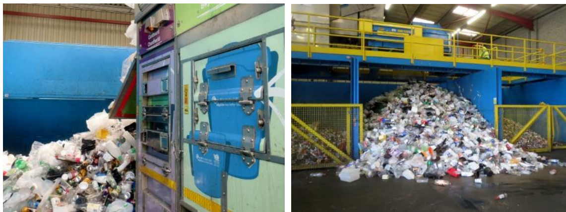
Figure 100: Sorting station – the plastic and metal packaging stream is sorted into three fractions
